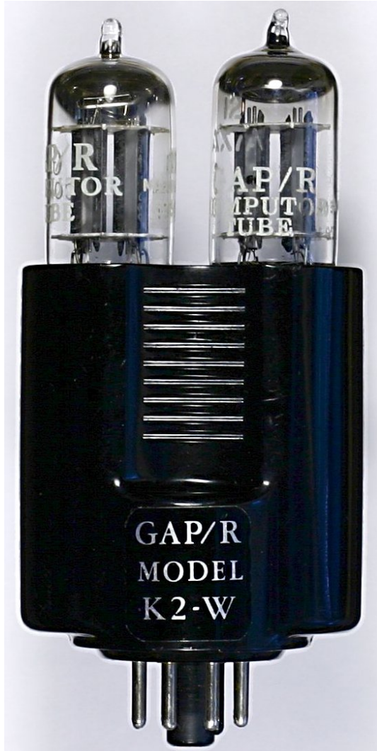
Vacuum tube operational amplifier, GAP/R K2-W, 1952
